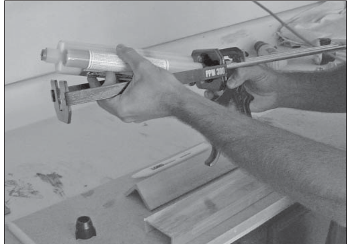
Loading cartridge into gun
