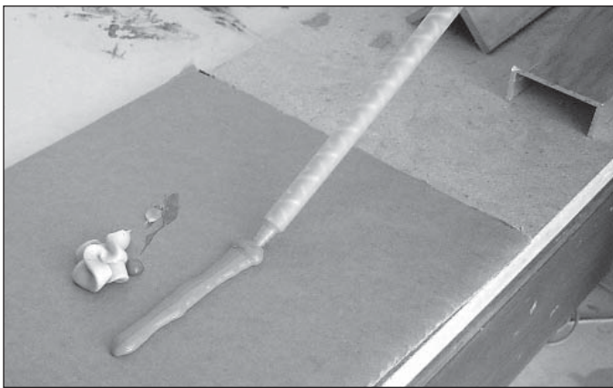
Dispensing adhesive through the static mix tip
