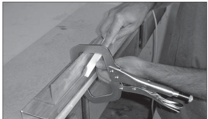
Removing excess adhesive
