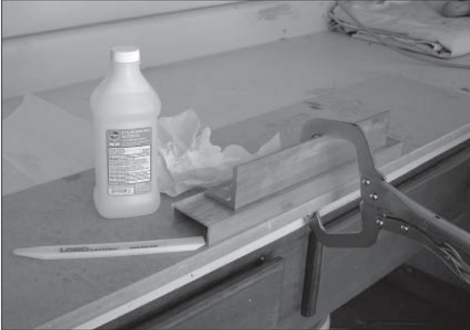
Rubbing alcohol removes smears or residue
