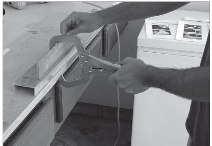
Clamping parts after adhesive application
